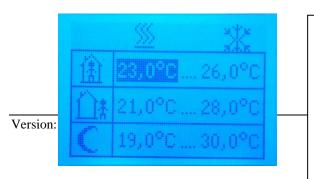
Adjust setpoint values for different operation modes and different control functions.
